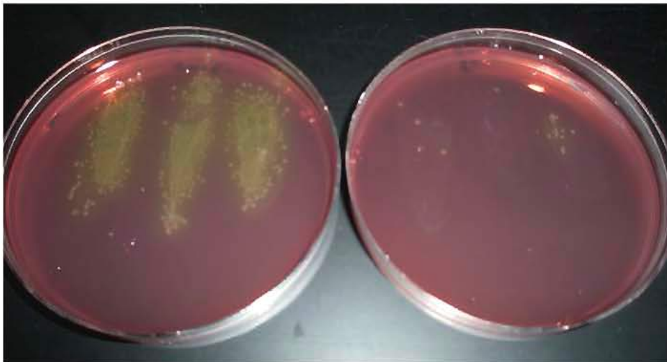
Left plate: control 3 logs of spores Right plate: Sterilray 13 spores, 1.1 logs of spores
