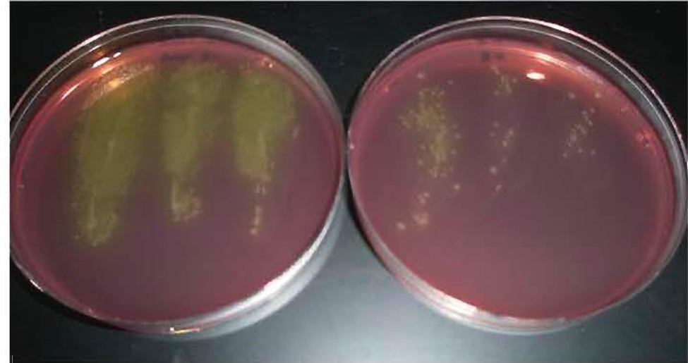
Left plate: control 4 logs of spores Right plate: Sterilray treated 60 spores, 1.8 logs of spores
